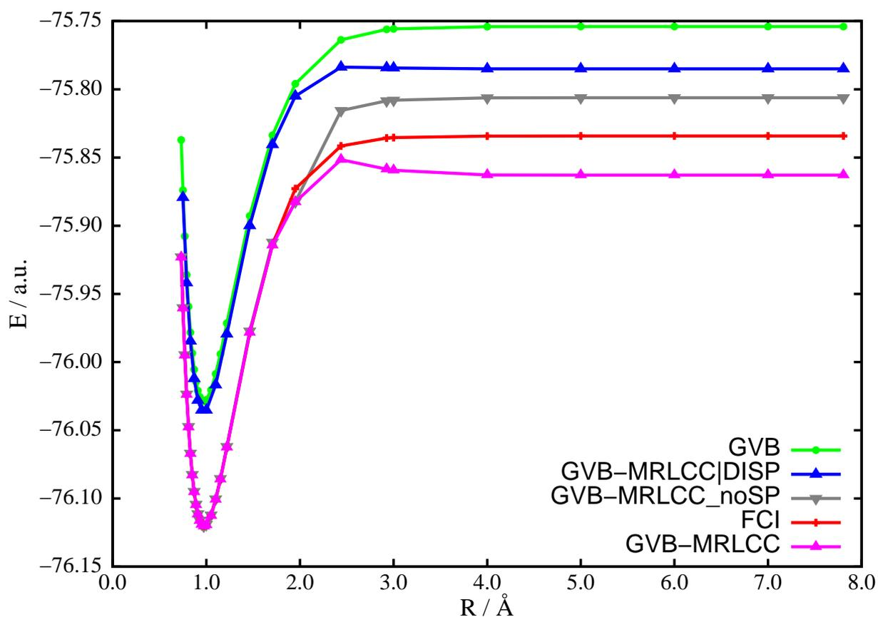
Figure 4: Water symmetric dissociation in 6-31G basis set with bond angle fixed at  $\angle(\text{H-O-H}) = 110.6^\circ$ . A GVB wavefunction is assumed as reference and frozen core approximation is applied. The GVB reference contains two orbitals on the bonding and one on the non-bonding geminals. See text for acronyms.
