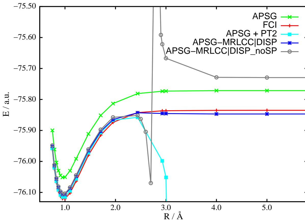
Figure 2: Water symmetric dissociation in 6-31G basis set with bond angle fixed at  $\angle(\text{H-O-H}) = 110.6^\circ$ . An APSG wavefunction is assumed as reference. Frozen core approximation is applied. The APSG reference has 4 orbitals on the bonding and 2 on the non-bonding geminals. See text for acronyms.
