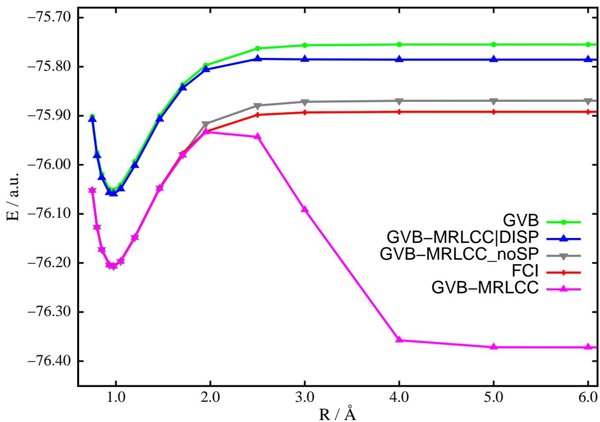
Figure 6: Water symmetric dissociation in 6-31G\* basis set with bond angle fixed at  $\angle(\text{H-O-H}) = 110.6^\circ$ . A GVB wavefunction is assumed as reference and frozen core approximation is applied. The GVB reference contains two orbitals on the bonding and one on the non-bonding geminals. See text for acronyms.
