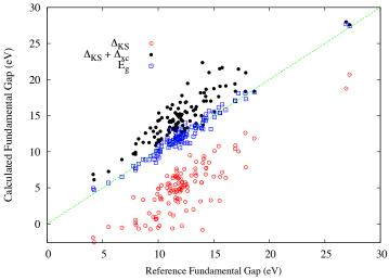
**Figure:** Calculated versus reference fundamental gaps for the FG115 database [2]. The fundamental gaps are calculated by three schemes (the KS gap, the KS gap + the approximate DD, the KS gap + the exact DD) using the LB94 functional [3].
