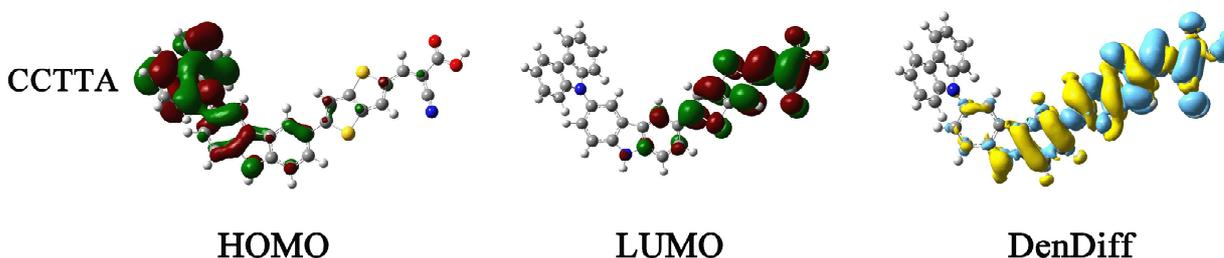
**Figure 1:** HOMO (left) LUMO (middle), and charge density difference (bottom) between the excited and ground states of the CCTTA dye.
