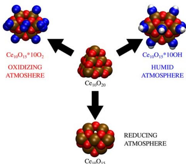
**Fig. 1** Our calculations predict that stoichiometric clusters have limited stability and readily transform into reduced clusters in oxidizing, humid and reducing atmospheres. This is exemplified in this figure for the  $\text{Ce}_{10}\text{O}_{20}$  (stoichiometric) and  $\text{Ce}_{10}\text{O}_{15}$  (reduced) clusters.
