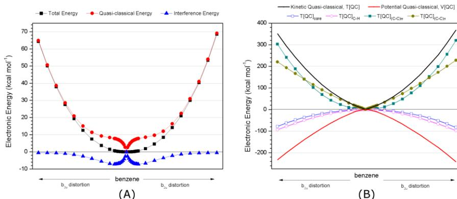
Figure 1 – Energy partitioning of benzene along the  $b_{2u}$  mode, obtained at the CASSCF(6,6)/cc-pVDZ level of calculation.
